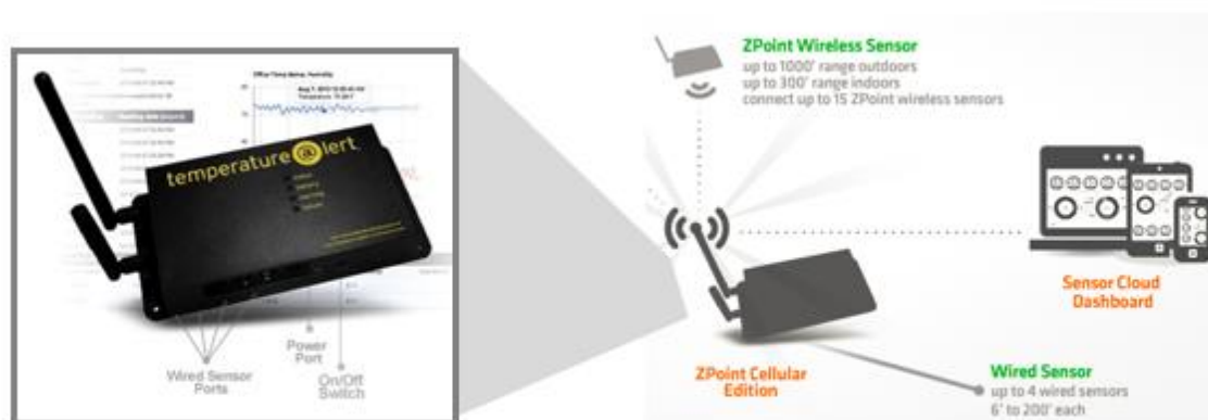
Figure F2: Temperature @lert temperature monitoring system
